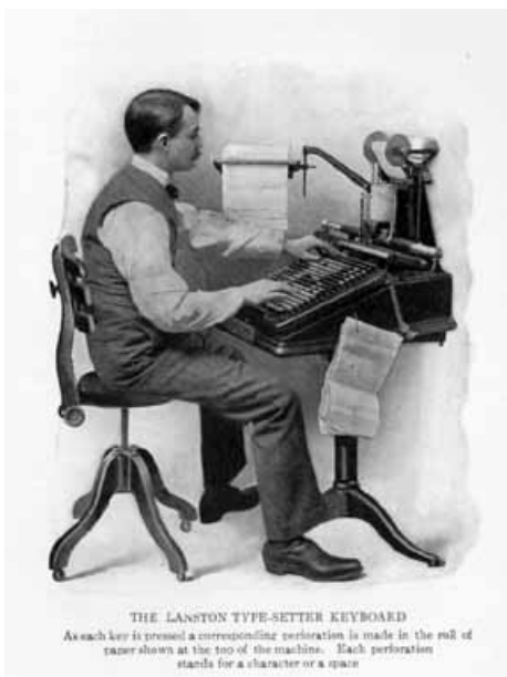
WHERE THE "BRAINS" ARE LOCATED The perforations in the paper ribbon (shown in the upper left-hand part of the picture) govern the action of the machine so that the proper characters are cast in their proper order, and also the spaces between the words
